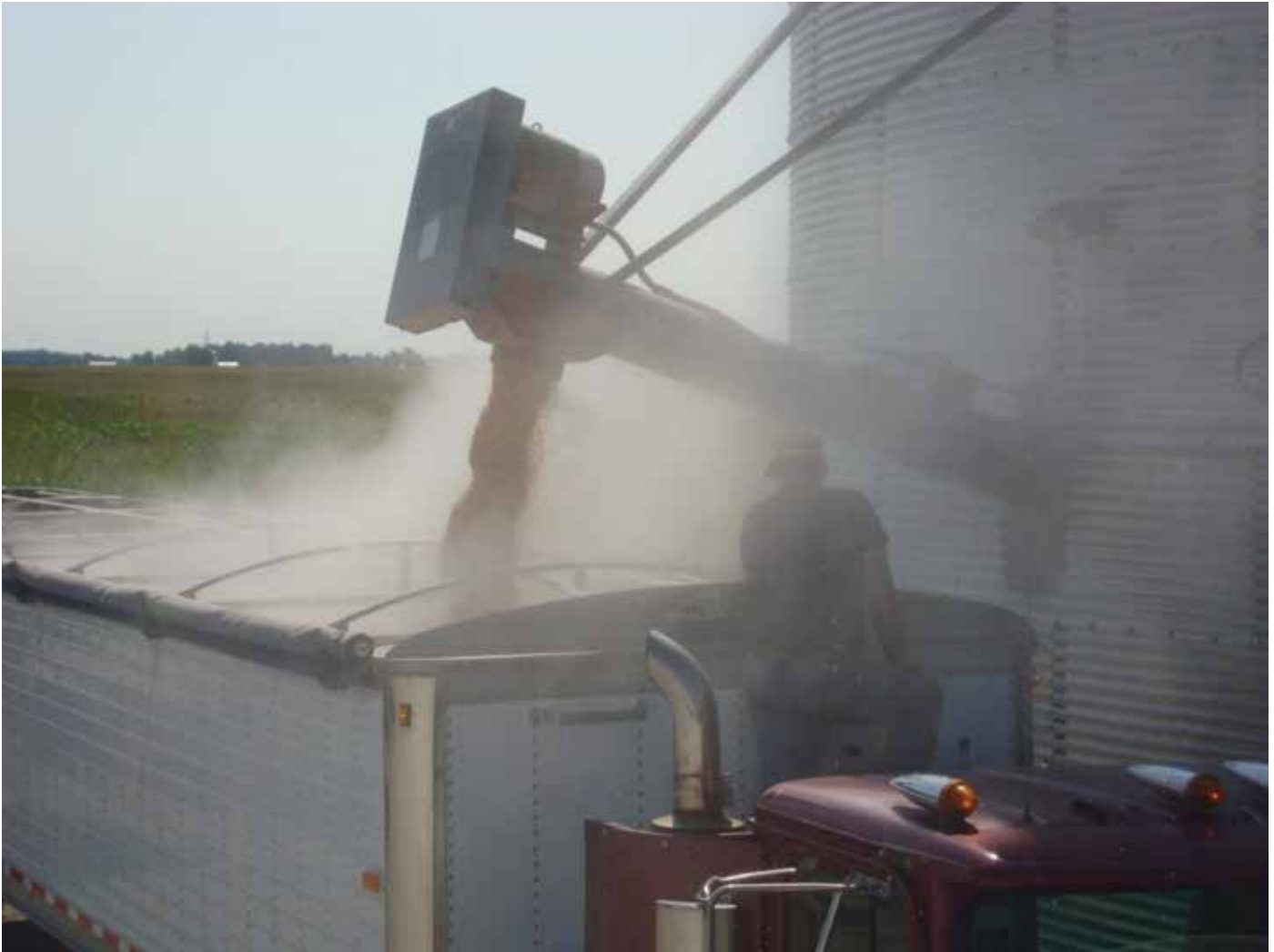
FIG. 1. Clouds of combustible dust are created when loading grain or processed meal into a bulk truck.
